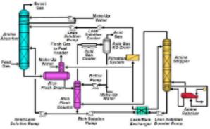
Raw natural gas streams often contain impurities that can cause significant damage to process, pipelines and equipment. Our acid gas removal solutions effectively remove hydrogen sulfide (H2S) and carbon dioxide (CO2) from gas streams to meet product specifications and protect downstream equipment.
